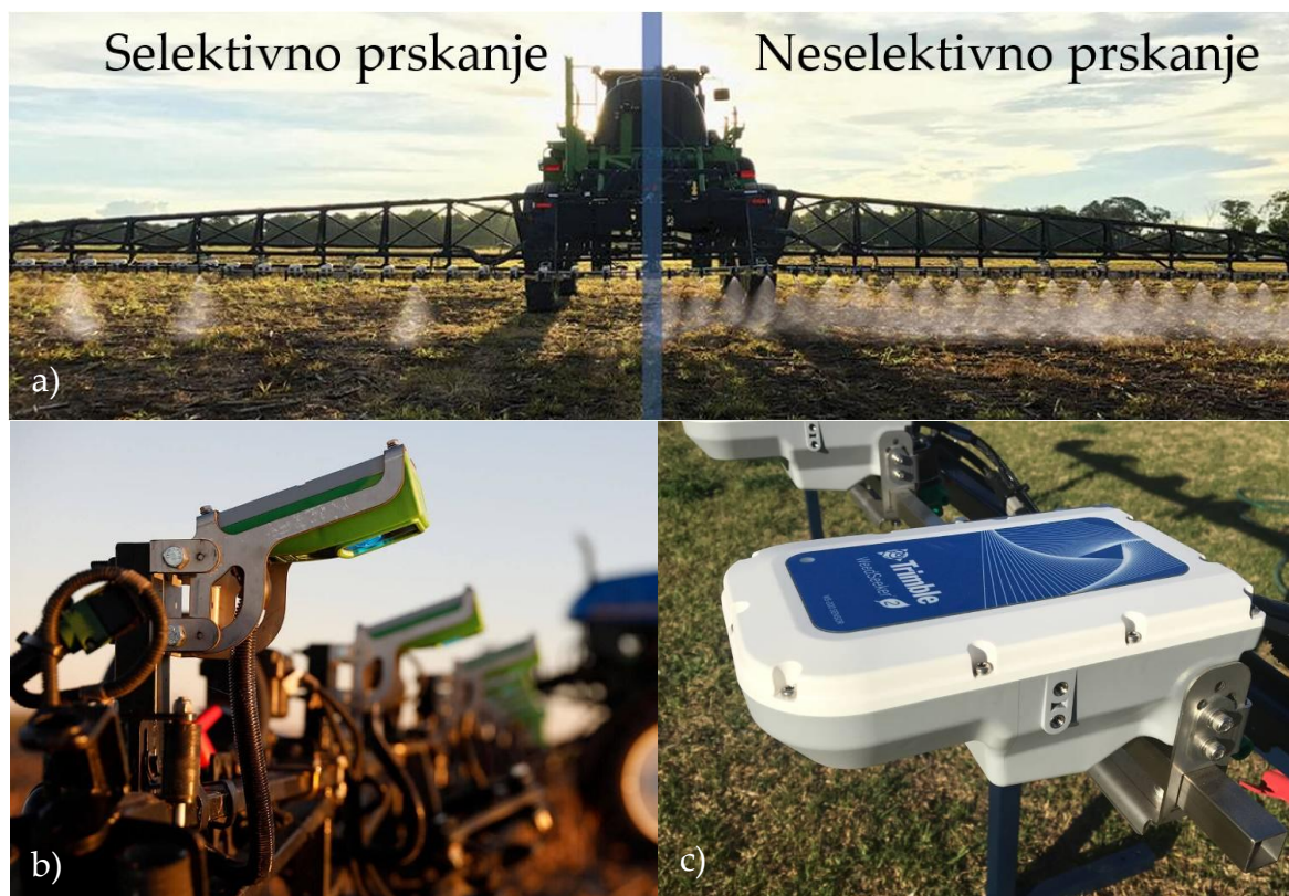
Slika 1.3. Koncepti primene pesticida (a); Weed IT (b) i WeedSeeker (c) senzori korova
